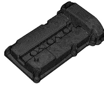
Figure 3a: A production engine valve cover model
